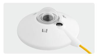
**CMP 6** is an ISO First Class pyranometer. It has a similar detector to CMP 3, but has improved performance due to the increased thermal mass and the double glass dome construction. The tilt error and levelling accuracy are also improved. The bubble level is visible through the snap-on white sun shield. The drying cartridge keeps the instrument free of internal condensation and is easily removable.
