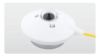
CMP 3 is an ISO Second Class pyranometer designed for shortwave global solar radiation measurements in the spectral range from 300 to 3000 nm. The thermopile detector measures irradiance up to 2000 W/m² with a response time less than 18 seconds and typical sensitivity of 10  $\mu\text{V/W/m²},$  that varies less than 5 % from -10 °C to +40 °C.
