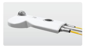
CNR 4 is a four-component net radiometer for accurate and reliable measurements and can be used as the reference instrument for a network of lower performance net radiometers. There are four separate signal outputs and the integrated temperature sensors can be used to calculate the FIR radiation. The screw-in mounting rod, bubble level, and cables with waterproof connectors, make installation easy.
