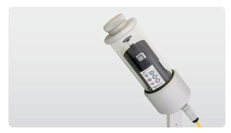
**CSD 3** measures sunshine duration through a high quality glass tube. It has no moving parts and uses 3 photo-diodes with specially designed diffusers to make an analogue calculation of when it is sunny. The output is switched high or low to indicate sunny or not sunny conditions. The calculated direct irradiance value is also available.
