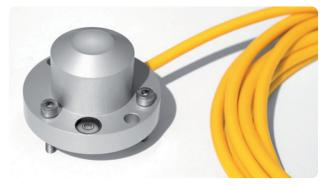
SP Lite2 is designed for all-weather measurement of solar radiation. It has a specially shaped Teflon™ diffuser that gives very good directional response and is largely self-cleaning. The detector is a silicon photo-diode, so the spectral response is not as broad or flat as our CMP series pyranometers with thermopile detectors. The standard cable length is 5 m with an option of 15 m.
