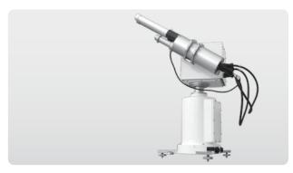
**POM-01** is a sky radiometer mounted on a dedicated sun tracker. It uses a single detector and rotating filter wheel to measure radiation in seven narrow wavebands, either directly from the sun or at user-defined angles away from the sun. The instrument has a base with levelling feet and a sun sensor for active tracking. Installation is quick and simple and a precipitation sensor is included so that the radiometer is pointed downwards during rain to keep the optics clean.
