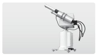
**POM-O2** has all the features of the POM-O1, but with extended waveband ranges. There is growing interest in monitoring aerosols of larger size and this requires measurement at longer wavelengths. In addition to the optical system with silicon photo-diode detector of the POM-O1, the POM-O2 has a second optical system with an Indium Gallium Arsenide infrared detector.
