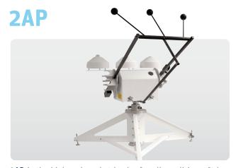
**2AP** is the high-end market leader for all conditions. It has proven performance in the harshest climates. High power motors and precision gear drives have the torque to break ice and to operate in high winds. Options enable operation down to -50 °C. After setup using Win2AP software and a PC, operation is stand-alone. The accessory heavy duty tripod stand provides a very stable mounting for the tracker.
