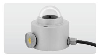
**CM 4** is a high temperature pyranometer for measuring solar or artificial light irradiance under the most extreme temperature conditions. With an operating temperature range from -40 °C to +150 °C and measurement up to 4000 W/m² it is a unique instrument. All the radiometer components are specially selected for their ability to withstand these extremely high temperature and irradiance levels.
