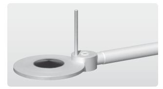
NR Lite2 is a single-component net radiometer widely used in agriculture and hydrology. The thermopile detector is fitted with black Teflon™ coated conical absorbers on both sides that have a very wide spectral response from the ultraviolet (UV) to the far infrared (FIR). The signal output is the difference between the sun and sky radiation and the ground radiation and can be positive or negative, depending upon the conditions.
